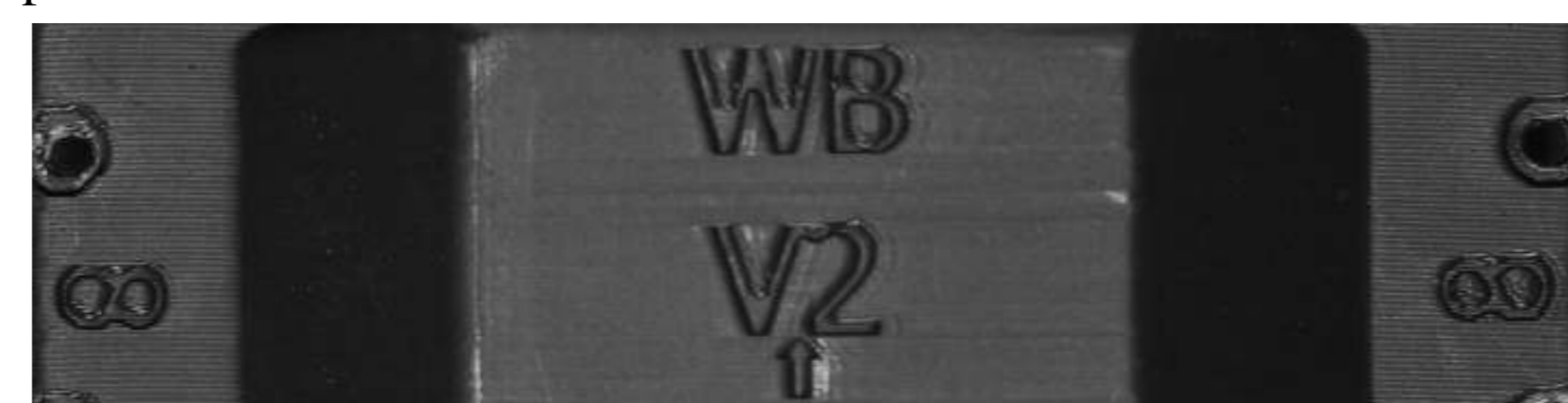
Figure 4: Example of a printed part with engraved information to simplify assembling. WB denotes the name of the part (waist bottom), V2 is the version, 8 indicates the required screw lengths (M2,5x8) and the little arrow shows the direction in which the part should be printed.
